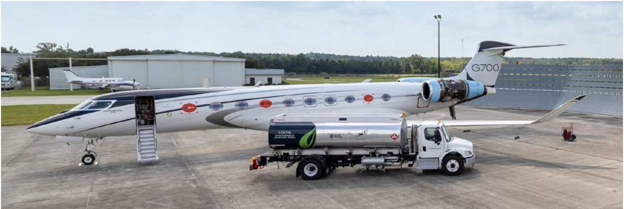
Gulfstream conducted ground emissions testing of 100% SAF from renewable feedstock in the Rolls-Royce Pearl 700, the engine designed exclusively for the G700 and G800. Preliminary results indicated minimal to no sulfur contamination of the fuel and the potential for reducing condensation trails and emissions.
