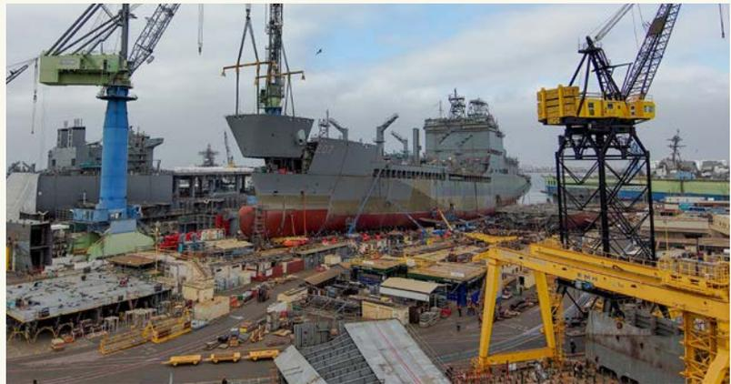
NASSCO has reduced its reliance on diesel equipment to decrease its emissions. The shipyard has more than 90 electric cranes and uses exhausted treatment systems and filters for equipment with large diesel engines. Since 2004, NASSCO has reduced overall diesel emissions by 80%. In 2022, NASSCO introduced a pilot program to use renewable diesel fuel in the shipyard that lowers particulates by 30% and reduces greenhouse gas emissions by more than 80% compared to traditional diesel fuel.
