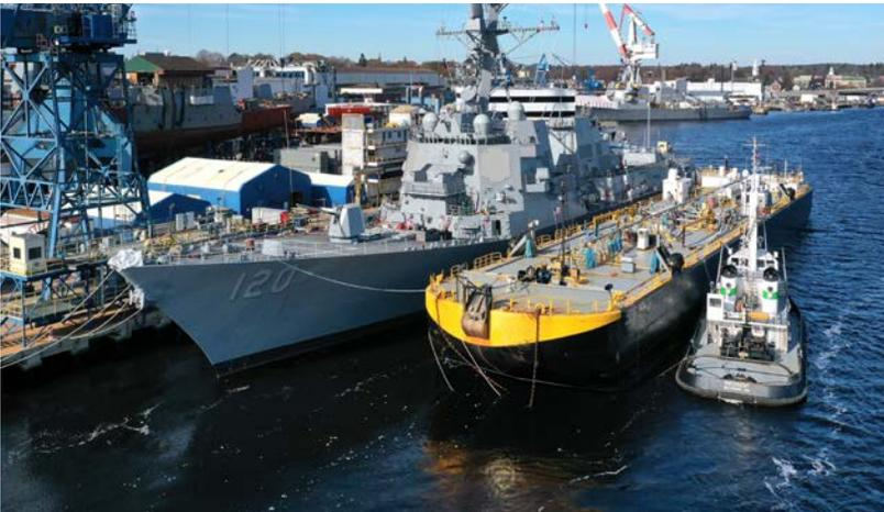
Bath Iron Works started using ocean barges instead of trucks to deliver fuel needed by its newly constructed ships for sea trials. What used to require 26 trucks, each making a 300-mile round trip from Boston to deliver fuel for a single destroyer, can now be accomplished with a single barge, reducing CO<sub>2</sub> emissions by 12 metric tons.
